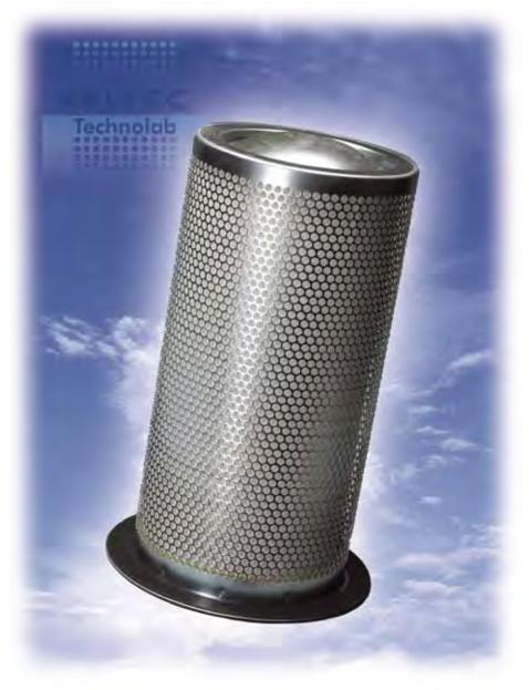
The standard conventional oil separator is the original design for the removal of oil aerosols from the compressed air stream. This element design consists of a specific amount of a uniform grade of borosilicate glass fibers, "wrapped" onto a support tube. When properly sized to the cfm/m3/ min flowrate and corresponding operating pressure of the machine, this element will provide consistent performance according to the following data:
