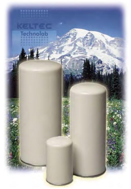
This method of oil separation consists of a deep bed type oil separator element, placed inside of a pressure resistant body, or "can" similar to that of traditional oil filters. Extremely easy to replace in comparison to standard oil-separators which are enclosed in a pressurized tank, this element design is somewhat limited in application due to restrictions of air flow capacity.
